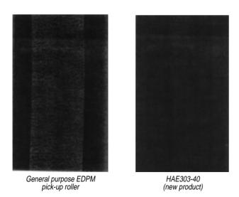
*Fig. 11 - Results of printing in the pick-up roller contact region No printing defects occur when using a feed roller made of HAE303-*40.
