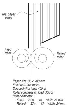
Fig. 2 - Retard roller accelerated paper feed test apparatus This test apparatus simulates the pick-up mechanism of office equipment such as photocopiers and laser printers, and allows such parameters as the feed rate and compression load to be set arbitrarily.
