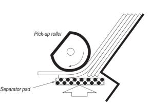
Fig. 9 - Separator-pad-type separator mechanism This is the separator mechanism currently used in most inkjet printers.
