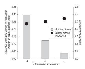
Fig. 7 - Relationship between vulcanization accelerators and wear resistance
