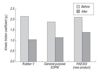
Fig. 12 - Change of  $\mu$  after feeding 2,000 sheets of coated paper A HAE303-40 is less susceptible to the reduction of  $\mu$  when using coated paper.
