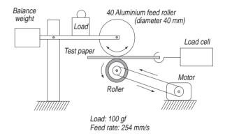
Fig. 3 - Friction coefficient measuring apparatus This apparatus can measure the coefficient of friction around the roller. The friction force is measured with a load cell and logged by using a recorder or a PC.
