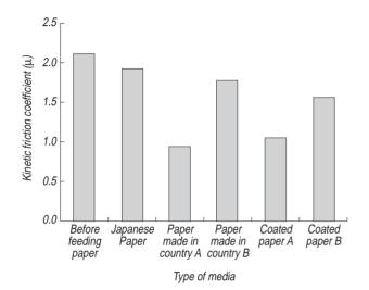
Fig. 1 - Changes in roller  $\mu$  with various types of media This graph shows how the friction coefficient of a "Rubber V" roller changes after feeding 2,000 sheets of each type of media. The reduction of  $\mu$  is particularly significant with plain paper made in country A and with coated paper A.
