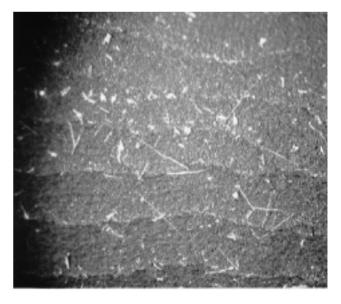
*Fig. 4 - Roller surface after feeding the paper made in country A The roller surface is covered with many needle-shaped paper particles, which greatly reduce the friction coefficient.*
